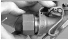
6. Insert the swivel into the coupler body until it is fully seated. A slight rotation assists with this assembly.
