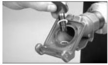
3. Put the o-ring over the disc stem. While holding the disc in the half turned position and taking caution not to scrape the disc edge against the coupler body, insert the disc stem into the stem seal and coupler body. Insert the disc until it is flush against the body.
