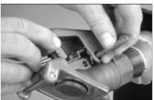
2. Pull the locking arm standoff out and remove the locking cap and locking cap spring.
