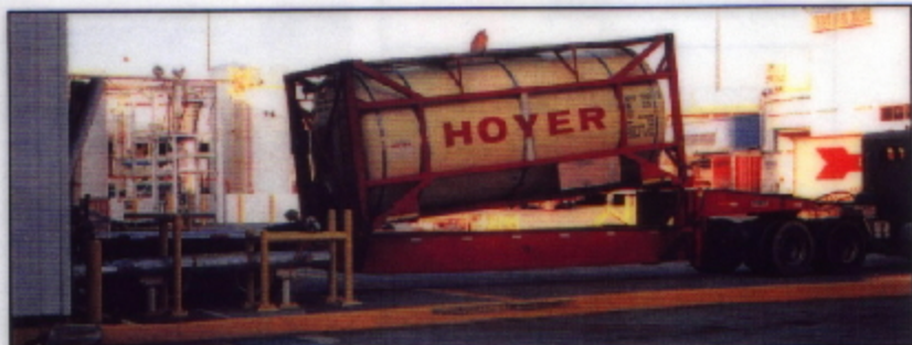
A container carrying laundry detergent ingredients is tilted for unloading at the Lever Brothers Company plant in Baltimore MD. The cargo is highly viscous.
